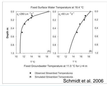
Example temperature profiles with fitted water fluxes
