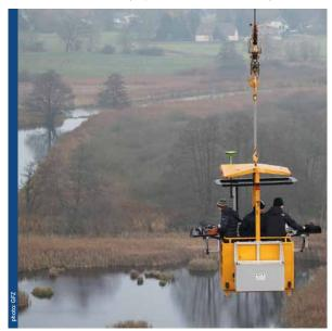
The crane serves as a universally applicable measuring station, which helps to close the gap between data recorded at ground level and from the skies. The Drönnewitz location is part of the DEMMIN test site, situated within the Neustrelitz site of the German Space Center (DLR), an important part of the TERENO observatory "Northeastern German Lowland".
