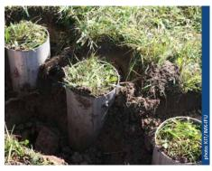
Climate simulation with small lysimeters
