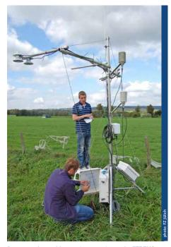
Important data: eddy covariance station at the TERENO Rollesbroich test site records latent and sensitive heat flow
