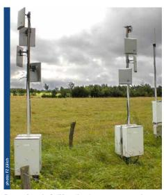
Routers from the SoilNet soil moisture sensor network at the TERENO Rollesbroich test site
