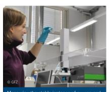
Measuring the stable isotopes of oxygen and hydrogen with the help of a cavity ring-down spectrometer
