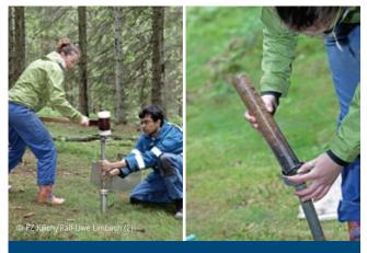
Collecting soil samples using a sample tube called a liner
