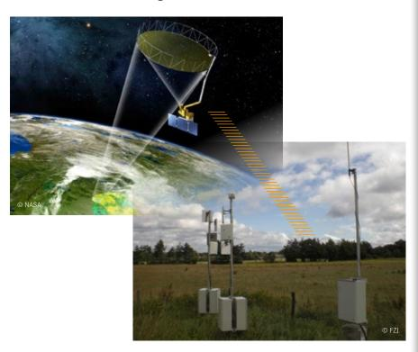
With the help of SMAP satellite data, researchers can generate very precise estimates of soil moisture content. Satellite data is compared with ground-based measurements taken at stations such as TERENO's Rollesbroich site.
