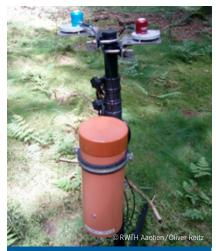
Tripod with PAR sensor (blue), R/FR sensor (red) and SoilNet data logger (orange).
