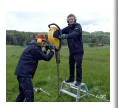
determining a location, for example, we use the signal that enters the sensor directly. But here we use the part of signal that first enters the soil and then the sensor. The signal changes depending on how much water is in the soil, and this allows us to draw inferences about the soil moisture," says Rasche.
