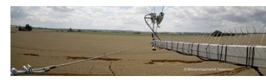
the help of a new radiometer. By combining state-of-the-art sensor and robot technology, they have ensured that high-quality in-situ measurements in all spectral bands – and for a broad range of water and land types – are available for validation of the surface reflectance data, which are needed to derive useful information from purely optical satellite missions.
