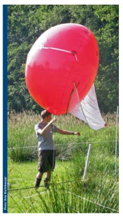
Just before lift-off: using balloons to measure air temperature
