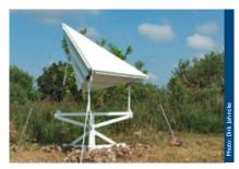
Signal exchange: corner-reflectors on the ground allow radar sensors to be calibrated
