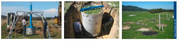
Installing a lysimeter: the openended cyclinder is filled with soil from the ground (left). Scientists then lift the full lysimeter out of the ground and insert the measuring devices (middle). When they are finished the only parts which are visible on the surface are air holes and lightning rods (right).
