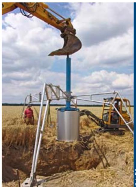
A lysimeter being filled with soil
