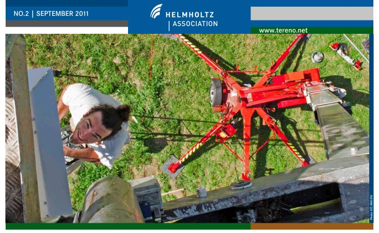
Aiming high: Christian Chwala from the Karlsruhe Institute of Technology (KIT) installs a self-developed measuring device at the Fendt test site that uses microwave radiation to test new methods for collecting precipitation and humidity data
