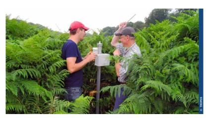
Near Jülich, TROPOS scientists installed roughly 100 pyranometers, which collect data on solar radiation levels.
