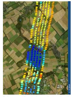
Radiometers provide precise data on soil moisture, but with low spatial resolution. Here, measurements are taken on a flight above the Blausteinsee lake near Jülich.
