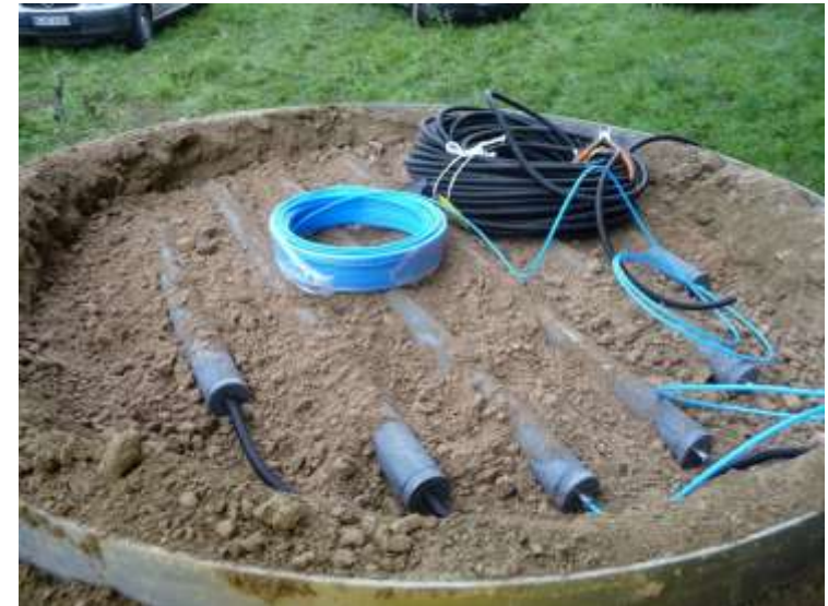
Suction cups rack as lower boundary condition
