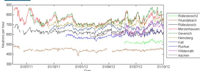
Fig. 3: Daily averaged neutron counts per hour corrected for pressure, incoming radiation and partially for absolute water vapor at ten locations in the Rur catchment normalised to sea level pressure (1013.25 hPa).
