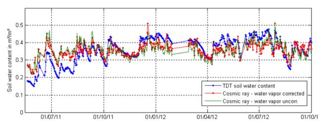
Fig. 6: Cosmic ray based soil water content and horizontally weighted soil water content of the TDT sensor network at the field site Rollesbroich for the whole measurement period. Visualisation of the benefits of water vapor correction by A(1) compared to no correction A(2) with RMSE and R<sup>2</sup> as in table 1.
