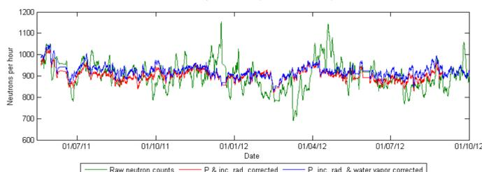
Fig. 4: 24 hour running mean neutron counts monitored by the cosmic ray probe in Rollesbroich: Raw counts, counts corrected for air pressure fluctuations and incoming radiation; counts corrected for air pressure, incoming radiation and water vapor in 2m height.
