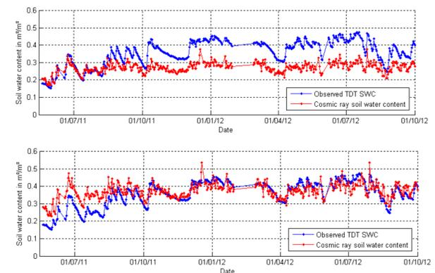
Fig. 7: Estimated soil water content and horizontally weighted soil water content of the TDT sensor network at the field site Rollesbroich for two shorter calibration periods: (B) 20th May – 20th Sept. 2011; (C) 20th Sep. 2011 – 7th Oct. 2012; R<sup>2</sup> and RMSE are for the calibration period respectively in as in table 1.
